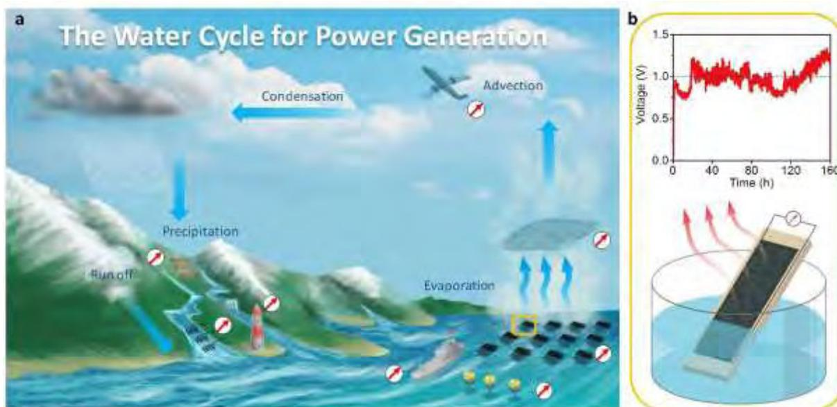
**Figure 2:** Harvesting the energy from the water cycle of the earth. (a) Devices for the energy harvesting(ref.6). (b) Electricity generation from natural water evaporation in ambient environment by carbon nanomaterials (ref.5).
